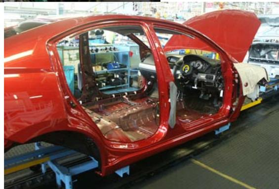
*Some of the last Mitsubishi 380 vehicles on the assembly line. Above, immediately after side panels had been attached to the chassis, and right, immediately after the dash panel had been installed.*
